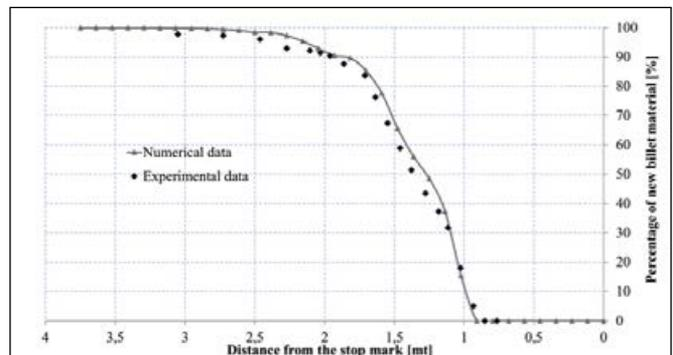
Figure 5. Comparison of experimental vs. numerical results for the percentage of new material over the stop mark distance for the extrusion of the structural profile shown in Figure 4.<sup>3</sup>
