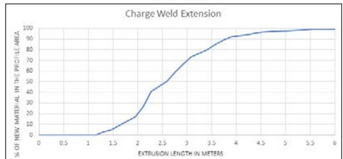
Figure 5. Example of the charge weld extension calculation by means of FEA, so that today the front-end defect can be known with high accuracy before the die is commissioned.
