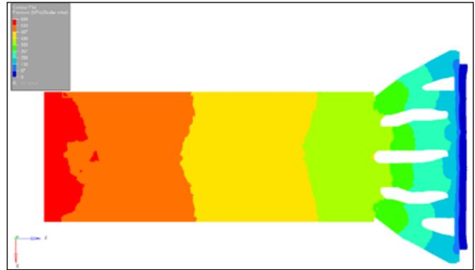
Figure 4. The press force required to extrude a defined billet length through the die is equal to the specific pressure at the dummy block times the container cross section area. In this case study the value is equal to 61 MN.
