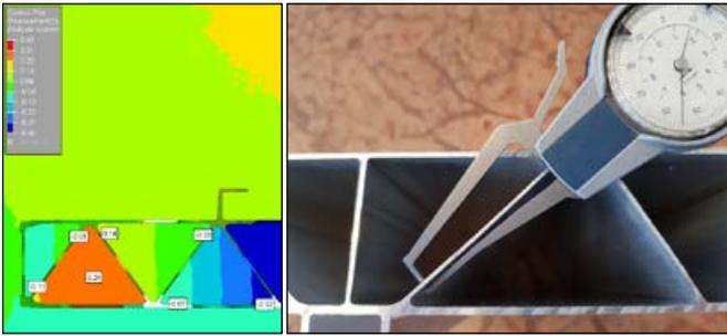
Figure 3. Prediction of mandrel displacement (vertical Y axis) in millimeters using an elastoplastic model (left). Dies that usually required correction at the vendor premises can be shipped overseas once it is verified that the wall thicknesses will be within tolerance, so that only minor corrections are required (right).
