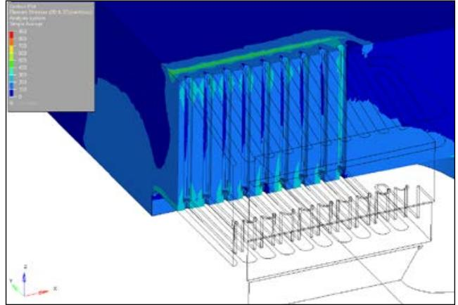
Figure 2. Stress analysis design by means of an elastoplastic model; today, the Von Mises stress, determined by FEA, is the critical factor affecting die performance.
